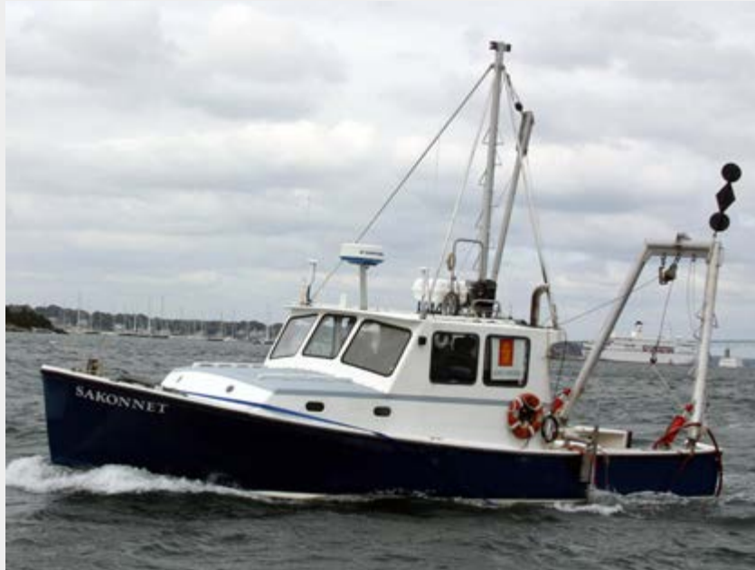
35-foot Bruno & Stillman fiberglass workboat outfitted for inshore survey and coring operations
