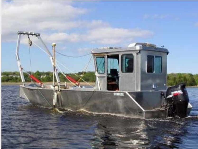
26-foot Stanley Bullnose aluminum workboat designed for inshore survey and coring operations
