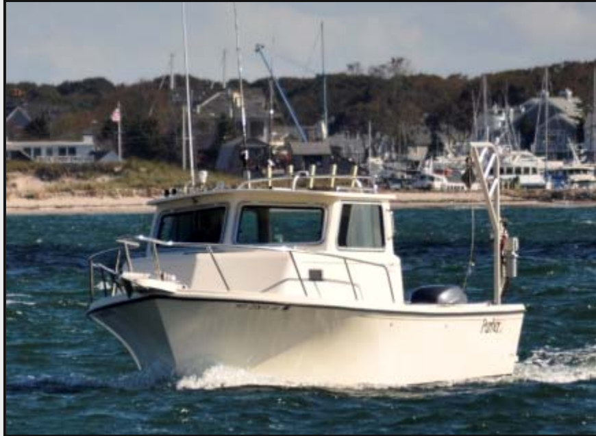
25 foot Parker fiberglass workboat designed for inshore survey operations
