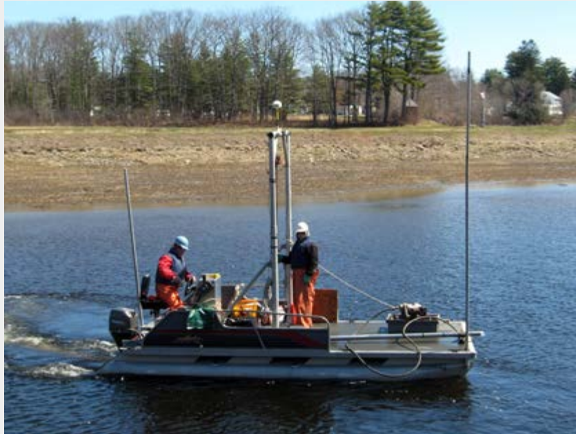
20-foot custom Pontoon Boat designed for shallow water vibracoring and sediment sampling
