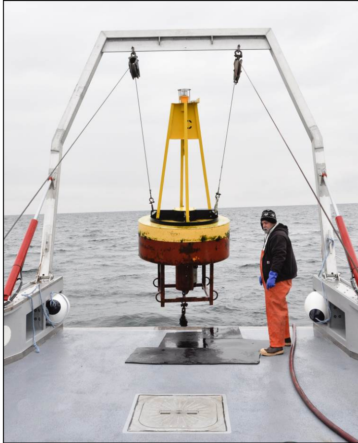
Maintenance of the Massachusetts DCR Cape Cod Bay Disposal Site buoy
